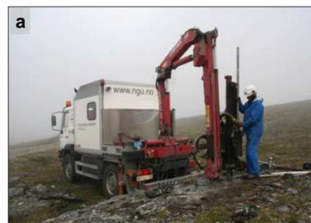
Figure 4. (a) Drilling of Lavkavagge 1 borehole, August 2007. (b) Temperature profile from Lavkavagge 1 borehole, recorded 07.09.2007. Seasonal frost reach a depth of more than 8 m.
